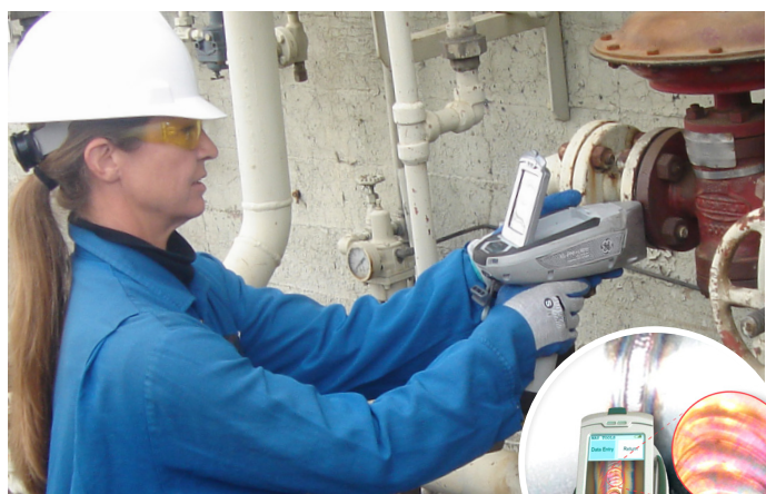
The CCD camera and WeldSpot small-spot focus feature allows isolation and analysis of weld beads and other small sample areas.
