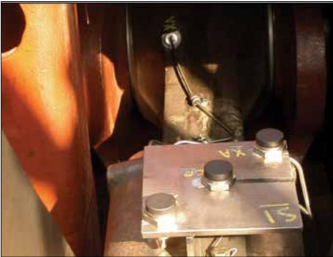
Figure 7. Wireless Temperature Sensors Installation on Connecting Rod.
