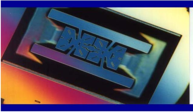
Fig 2 GE Druck RPT single crystal silicon element.
