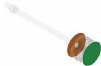
Figure 2. Piston areas used for gas rod load calculation
