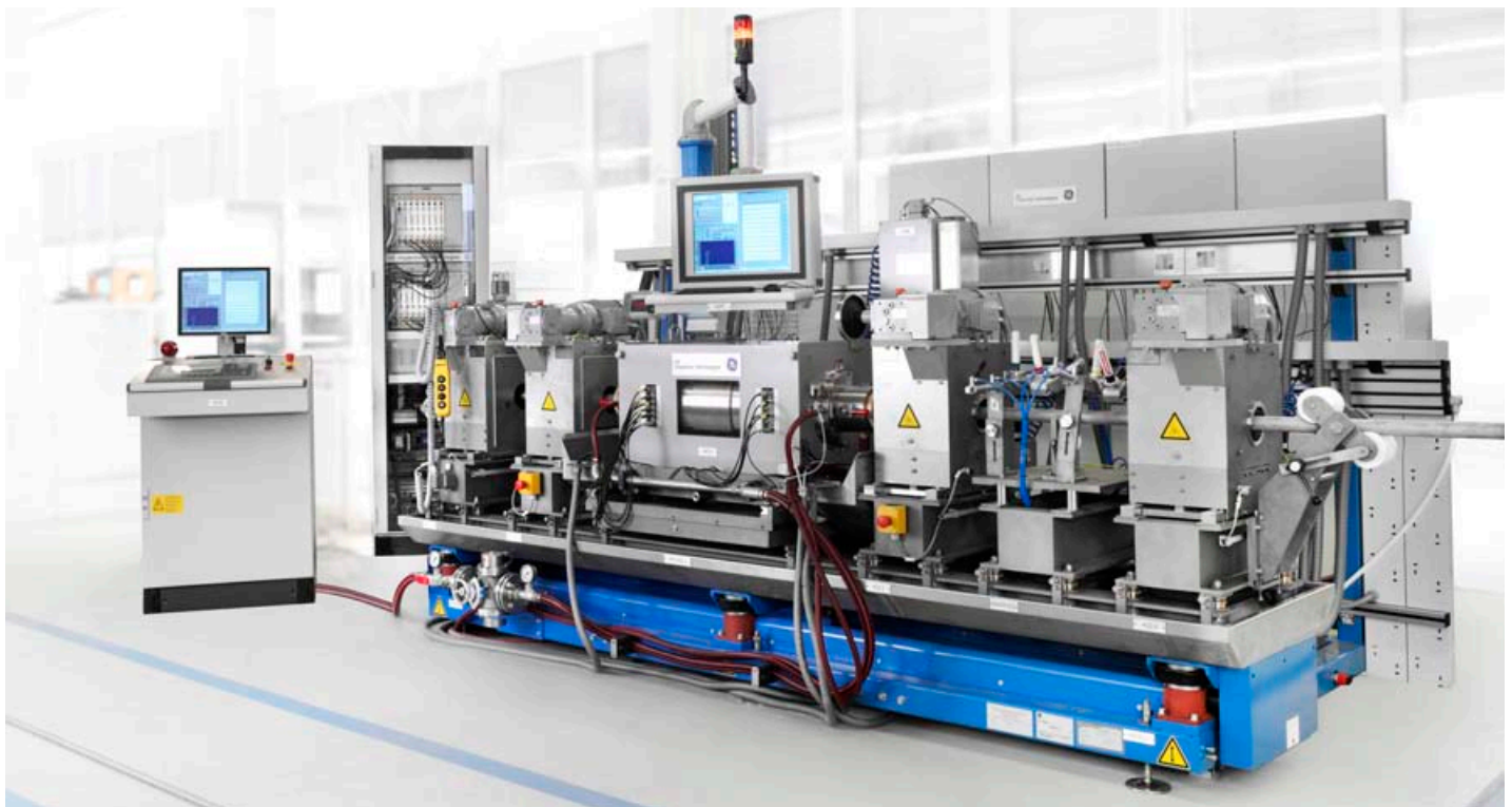
Ultrasonic tube testing with rotating probe system
