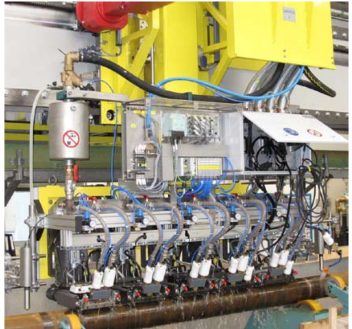
Ultrasonic tube testing with scanner technique
