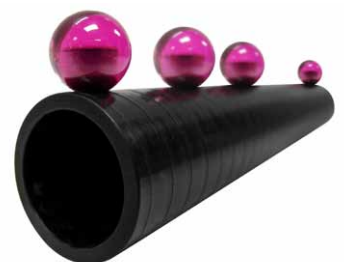
Measurement of sphere distances with a calibrated test specimen and comparison to the calibrated values
