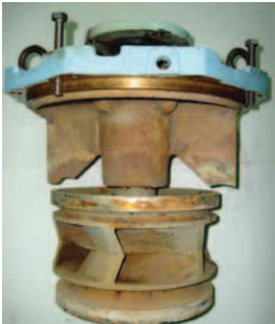
Figure 4: Pump internals after removal for inspection. Observe the significant loss of metal from the tips of the casing flow vanes (fins). Approximately 19 mm of metal was lost in two places. Fin thickness was also reduced from the original dimension of 7 mm to 4.5 mm. It turned out that the Vane Pass anomaly was produced by this damage, rather than by deterioration of the impeller.
