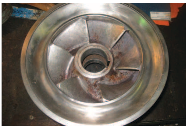
Figure 6: Impeller after cleaning. Axial view into one of the impeller eyes (suction).
