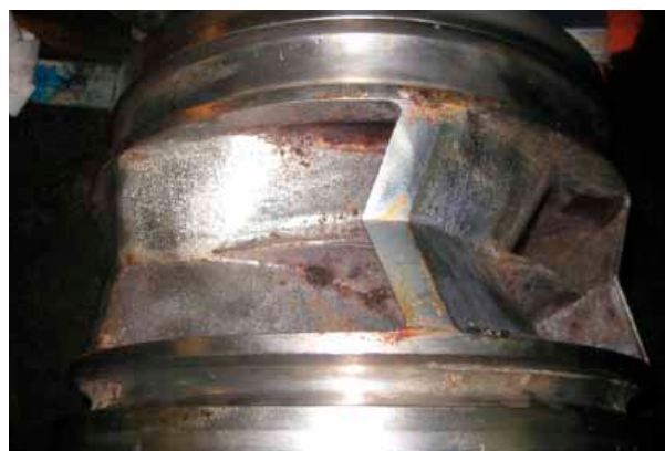
Figure 7: Impeller after cleaning. Radial view of the impeller vane tips (discharge).
