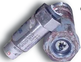
Figure 1 – Broken cylinder pressure transducer due to inadvertent contact with an overhead crane hook.
