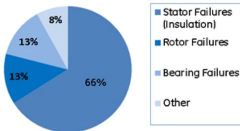
Understanding how motors fail helps point to a solution. If a technology exists that allows owners and operators to track the insulation degradation online reliably over time this would prove a useful tool. Outages could be scheduled and unplanned events could be avoided, Yielding increased reliability and safety.
