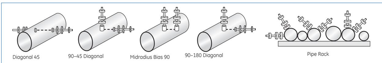
Standard transducer mounting configurations
