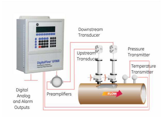
Typical meter set-up for standard volumetric or hydrocarbon mass flow
