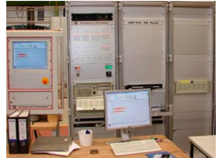
Back end electronics with realtime event LED panel
