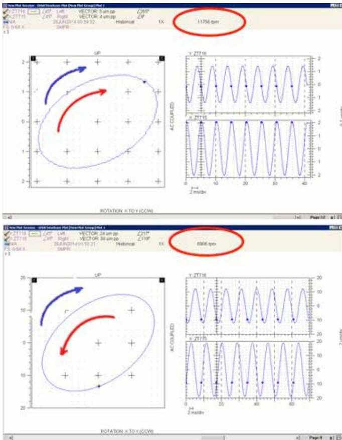
Figure 9: 1X- filtered orbit plot before and during the shutdown event
