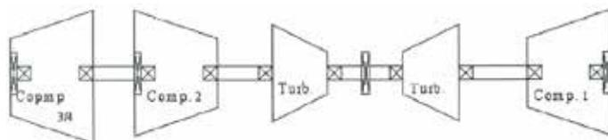
**Figure 1: Turbine-driven compressor machine train**
