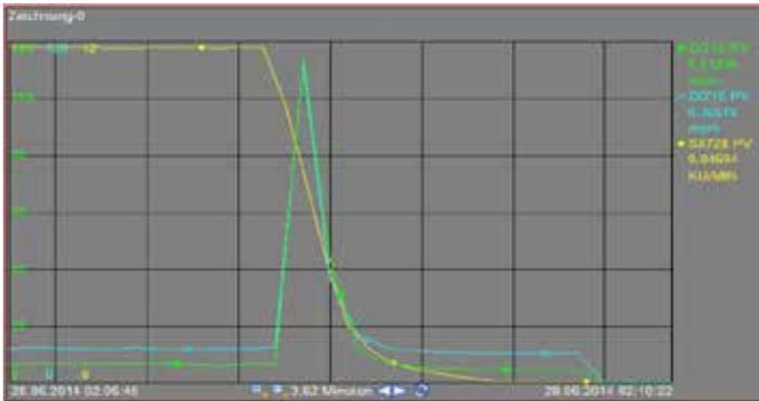
**Figure 5: DCS reading of the event** (yellow line indicates turbine operational speed, blue/green lines indicate vibration level in  $\mu\text{m}$ )
