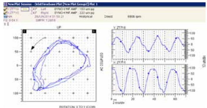
**Figure 8: Orbit plot during shutdown**
