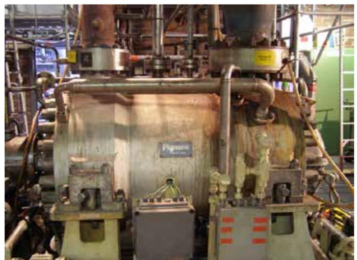
**Figure 4: The high pressure compressor that is part of the machine train**
