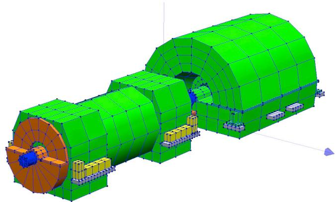
**Figure 1.** Example of ODS for Structural Vibration Study of an LP Turbine and Generator
