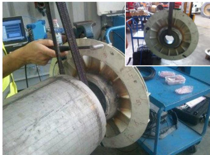
**Figure 2.** Example of Modal Impact Test on Machine Section
