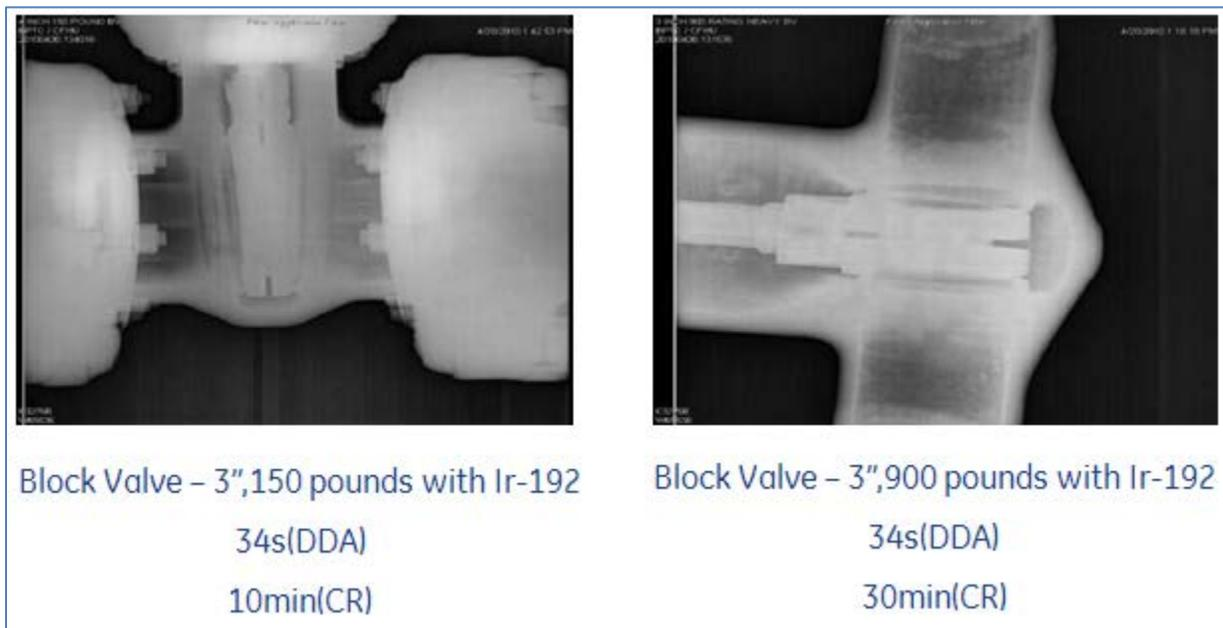
Figure 1: Two application examples showing comparing DDA and CR exposure times
