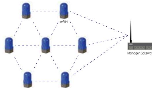
In a mesh network, each device is a peer that can talk to other peers, resulting in multiple signal transmission paths, higher reliability, and higher deployment flexibility.
