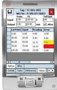
Failed calibrations will trigger a deviation in the field and force the technician to enter details of the failure for others to investigate after notification.
