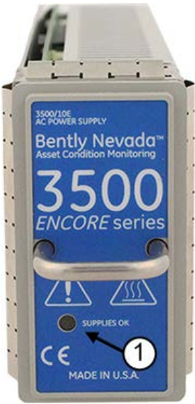
Power Supplies OK LED
